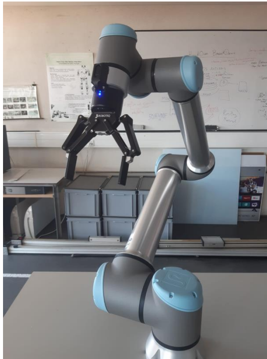
Figure 5 - UR10e collaborative manipulator with adaptive gripper 2F-140, installed in the LARCCell
