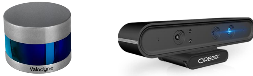
Figure 10 - Velodyne VLP16 and Orbecc Astra Pro camera.
