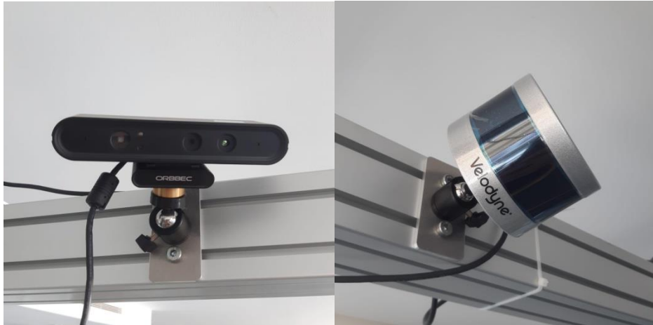
Figure 14 - Velodyne and Orbecc Astra Pro installed in the collaborative cell
