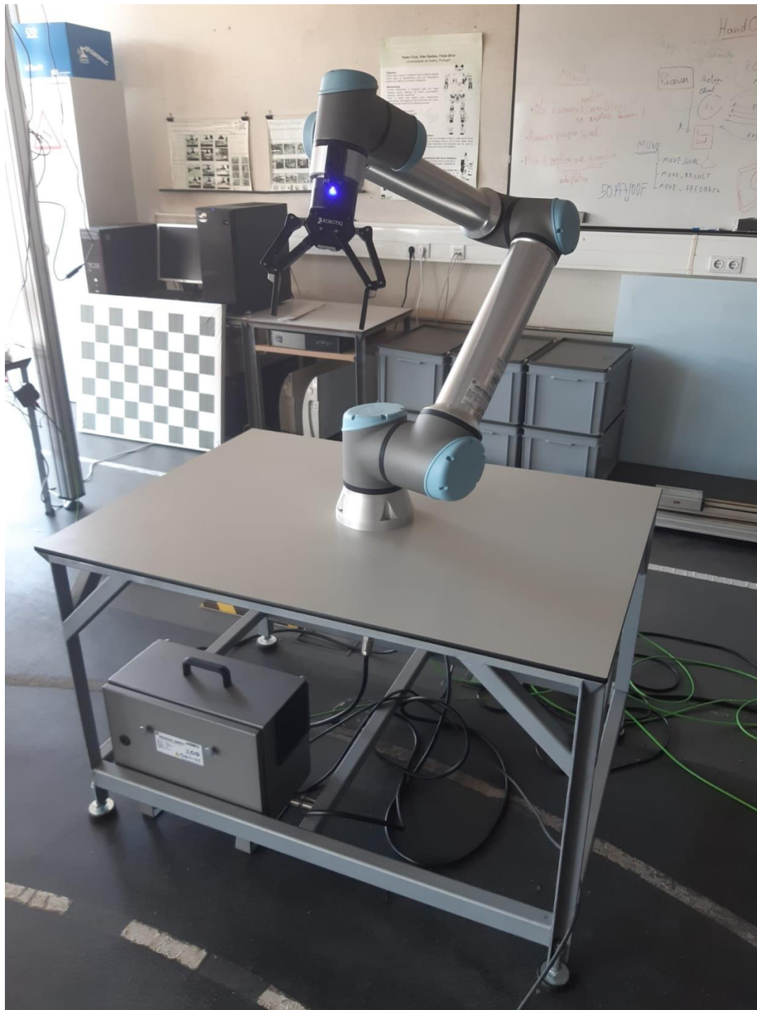
Figure 9 - UR10e manipulator and 2F-140 gripper, mounted on the support in the collaborative cell.
