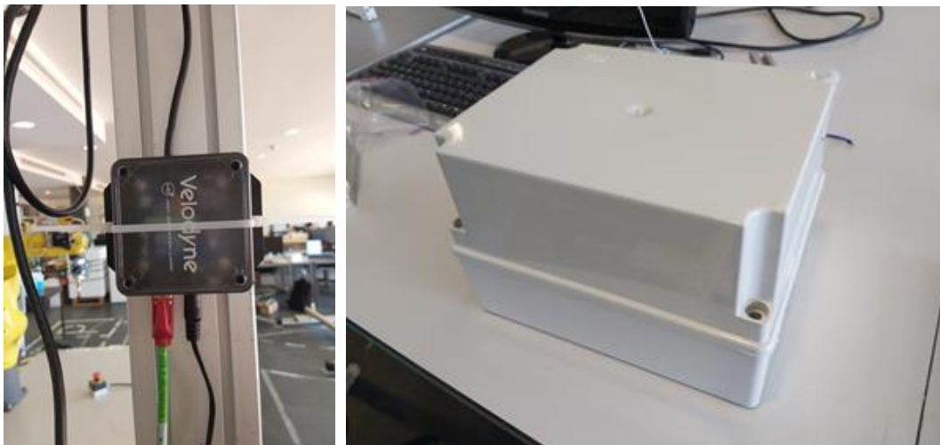
Figure 32 - Connection box of a Velodyne detector and the respective encapsulation box
