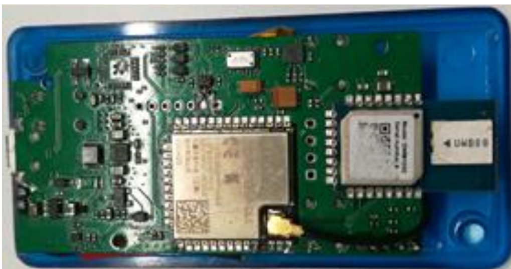
Figure 2 – 5G Tag first prototype.
