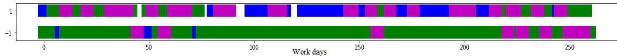
Figure 7 – Influence level of the OEE factors throughout the workdays - (blue) is the positive/negative Availability influence; (green) is the positive/negative Performance influence; and (purple) is the positive/negative Quality influence. Positive influence has the value +1 and negative the value -1.
